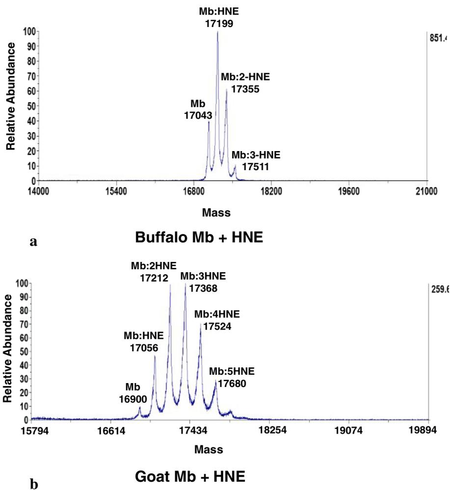
**Fig. 7** MALDI-TOF MS spectrum of (a) buffalo meat oxymyoglobin (0.15 mM) reacted with HNE (1.0 mM) and (b) goat meat oxymyoglobin (0.075 mM) reacted with HNE (0.5 mM) at pH 7.4 and 37 °C for 3.5 h
